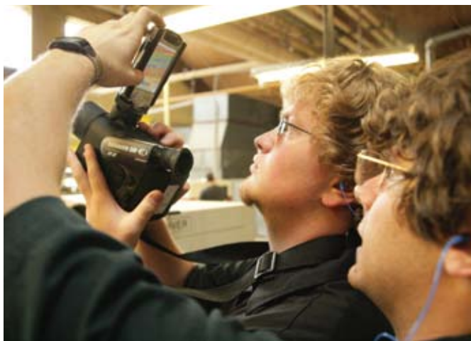
Students use a thermal-imaging camera to measure the efficiency of the factory's lights.
